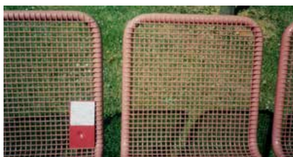
Fig. 5.1.1 Not sufficiently resistant to cleaning agents
