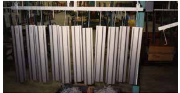
Fig. 2.4.2 Incorrect positioning of workpieces
