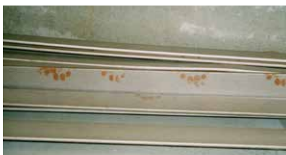
Fig. 3.8.2 Contamination due to hand sweat, hand cream, ...
