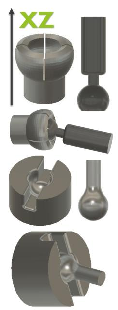
It can be tricky to get the dimensions between the ball and the socket right at first - always test your design before printing a high quantity.
