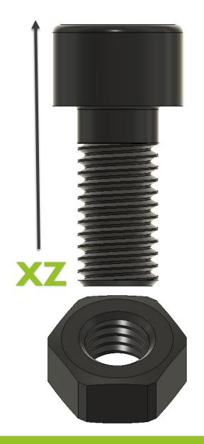
It is not recommended to print threads with a pitch smaller than 1 mm.
