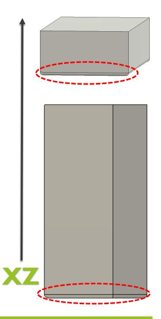
Generally, it is recommended to orient important features that need high accuracy and good resolution facing upwards.
