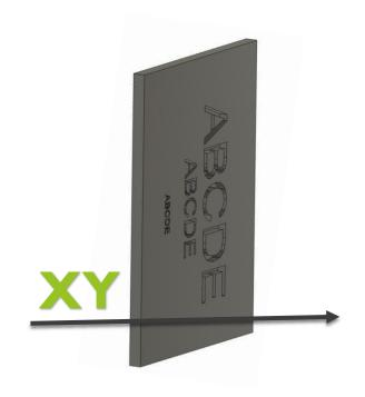
The sweet spot for engraved features is an engraving depth between 0,75 to 2 mm and a lettering height of at least 4mm.
