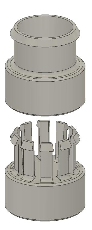
Annular snap fits are not suited for very rigid materials. A viable alternative is segmented annular snap fits that work on the principle of a flexural beam.
