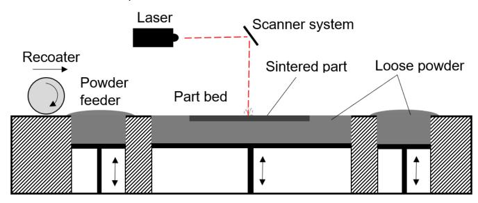
As soon as the printing is finished, the material needs to cool down. As a rule of thumb, conventional SLS materials (like polyamide) require a cooling time similar to the printing time. One of the benefits of thermoset polymers is a reduced cooling time – typically **half of the printing time is sufficient**.
