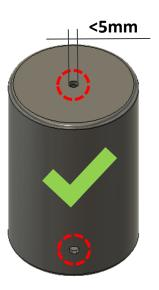
Be cautious if using compressed air to clean a cavity with only one escape hole of a small diameter (< 5 mm), the pressure may cause the part to burst!
