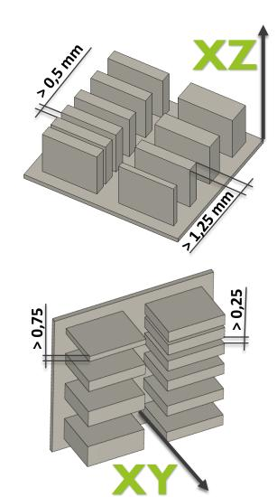
Delicate ribs can be especially difficult to depowder. Due to the large surface area they tend to snap off easily if you blow compressed air directly at them.
