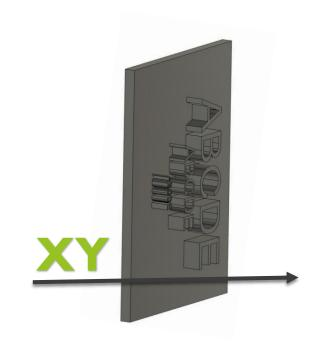
The sweet spot for embossed features and lettering is a protrusion height between 1 to 2 mm and a lettering height of at least 4mm.
