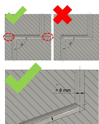
The smallest angle and diameter of the interconnection between the entry and exit holes that is possible to depowder without the use of escape holes is at least 110° with a diameter of at least 8 mm.
