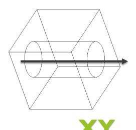
If a perfectly round hole is required by default, place the hole in the XZ direction.
