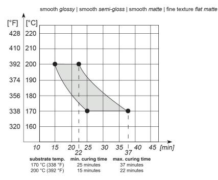
Cure parameters must be closely observed since mechanical properties will develop before full cross-linking.
