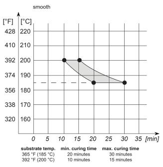
Cure parameters must be closely observed since mechanical properties will develop before full cross-linking
